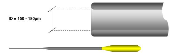
3. <u>Manipulation (blastocyst) pipette:</u> (blunt opening) Is intended for manipulation of human embryos in the stage of expanded resp. hatching blastocyst
