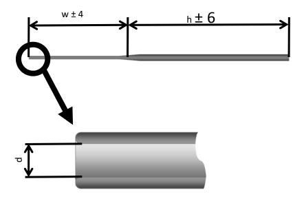
Currently manufactured intended lengths  $\underline{w}$  are as in the table below. Please mind that the length may however vary in a tolerance of few millimetres.
