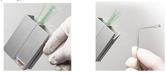
The cutting procedure is shown in the picture above. First, pull the straw down through the gap in the SG Cutter. It is important to hold the straw close to the cutter to protect the capillary inside. Bend the cut-off part on the top of the straw.
